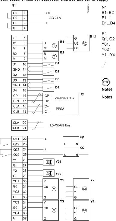
RXC39.5 LG-Ni 1000 temperature sensor Air quality sensor (DC 0...10 V) Volt-free contacts
